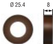
Ring magnet Part No. 400533 OD 25.4 mm ID 13.5 mm Height 8 mm Surface pressure max. 40 N/mm 2 * in axial direction
